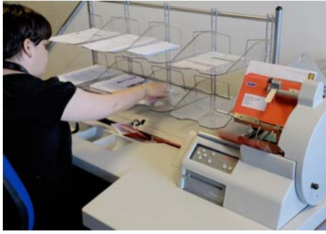
The centre is equipped with an Opex 51 Rapid Extraction Desk (pictured) and a Twofold 606e high-speed mail opener.
